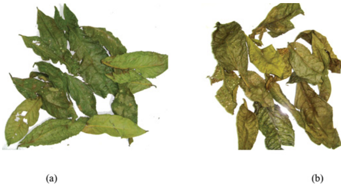
FIG. 11. Color parameter of the tea leaves dried in microwave operation mode (vacuum pressure of 385 torr, microwave power of 800 W): (a) pulsed microwave operation mode and (b) continuous microwave operation mode (color figure available online).
